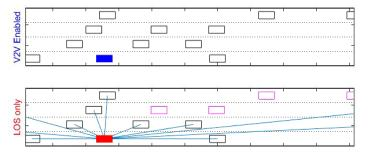
Red: LOS only Ego Vehicle Blue: V2V enabled Ego Vehicle Black: Currently detected vehicles Magenta: Current undetected vehicles Line segments: vehicles detected via LOS sensing
